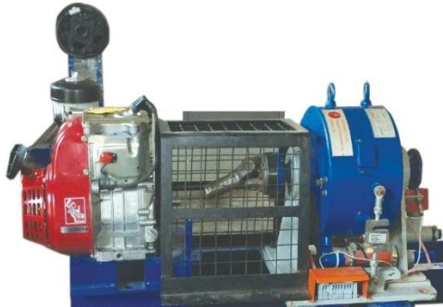
FIC 101 A SINGLE CYLINDER FOUR STROKE PETROL ENGINE WITH EDDY CURRENT DYNAMOMETER
