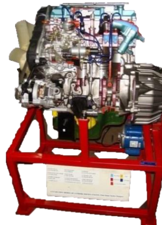
FICM 205 ACTUAL CUT SECTION OF 6 CYLINDER 4 STROKE PETROL ENGINE MOTOR DRIVEN
