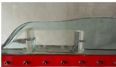
BROAD CRESTED WEIR
