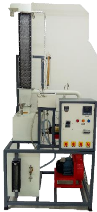
FHT 309 WET COOLING TOWER
